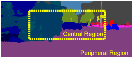
Figure 5: Typical parsing result of baseline FCN model. We evaluate FCN on peripheral and central region respectively, to analyze how much a perspective distortion affects urban scene parsing.
